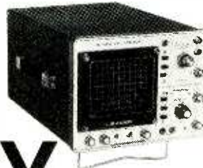
LBO-502 — 5" Solid State Triggered Scope
